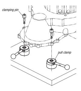
Simultaneous clamping and positioning of a workpiece
