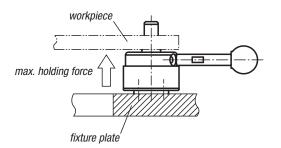
Make sure that no force exceeding the values in the table is affecting the bottom of the workpiece.
