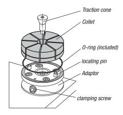
2.2 Machine the contour of the part that is to be held into the collet.
