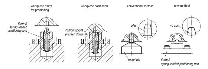
The conical spigot is pushed down when the workpiece is mounted on the positioning unit.
