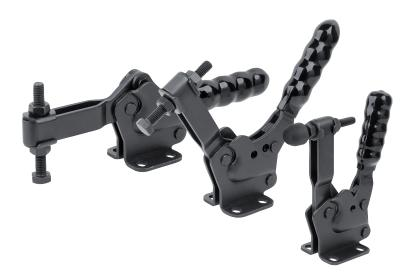
Toggle clamps generate the maximum clamping force when the three pivots are in a straight line (dead centre position). A clamp is locked by moving one pivot beyond the dead centre position. The end position over dead centre is carefully chosen to retain the maximum clamping force while preventing inadvertent opening of the clamp due to vibration or varying loading.
