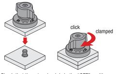
Check that the rotary knob is in the "OFF" position. Set the quarter-turn latch over the clamping pin and turn the rotary knob to the "ON" position. When fully clamped, a click sound is heard.
