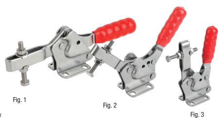
Toggle clamps generate the maximum clamping force when the three pivots are in a straight line (dead centre position). A clamp is locked by moving one pivot beyond the dead centre position. The end position over dead centre is carefully chosen to retain the maximum clamping force while preventing inadvertent opening of the clamp due to vibration or varying loading.
