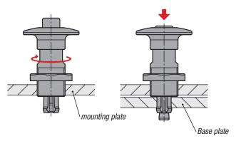
Screw the locking pin into the mounting plate until the thread can be seen on the other side.
